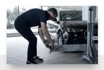
Adjust the cross member (up to 1 m) to correspond with the radar calibration.
