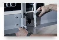
Lift or lower the panel for a parallel alignment by means of a lever.
